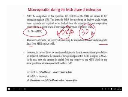
So, in the third stage it says that the memory buffer register will write to the instruction register. So, if it an immediate data more or less our job is done, because now your instruction register basically has the memory buffer register which is having the data called ADD accumulator 30 H which is a may be immediate.
