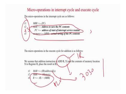
So, in the from the instruction register you have to get the value of X. Address X means the value of X that is 3030 in the example we are looking at. So, memory address register will be fed with the value of address of X.
